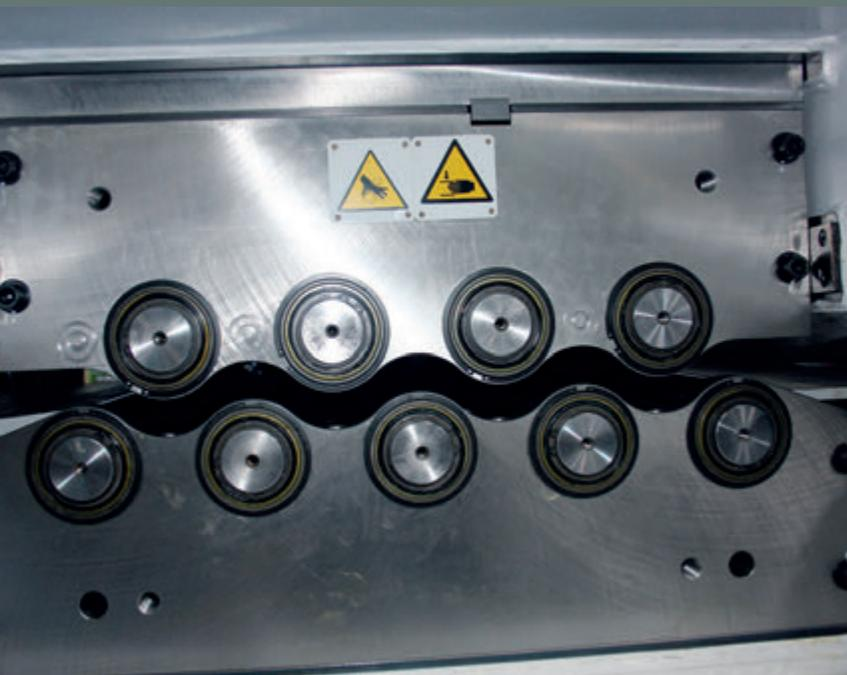
*the necessary planarity to the material" Crespi explains. It is interesting to note that in this case, although the material is rather difficult and demanding, the number of rollers used is low because the planarity needed by the client did not require a larger number of rollers, so the costs were not unnecessarily increased.*
