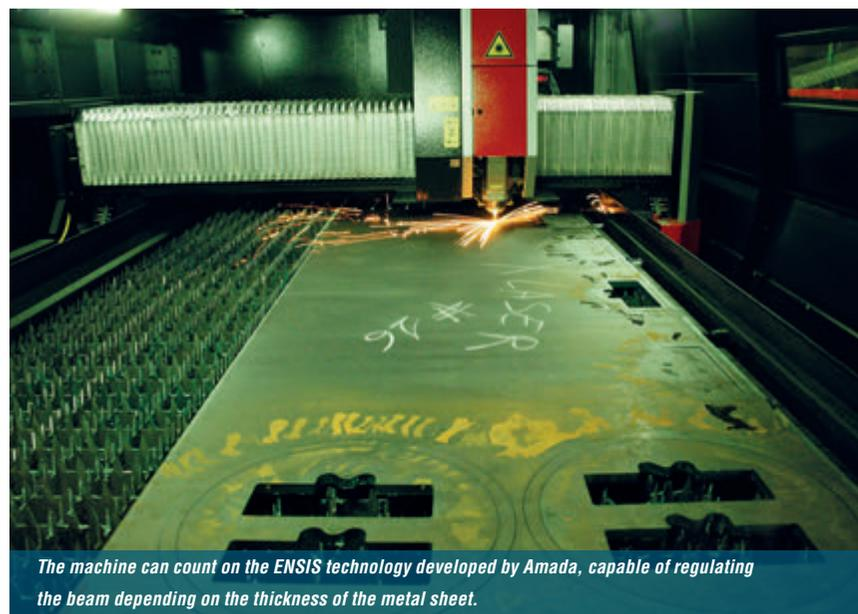
The machine can count on the ENSIS technology developed by Amada, capable of regulating the beam depending on the thickness of the metal sheet.
