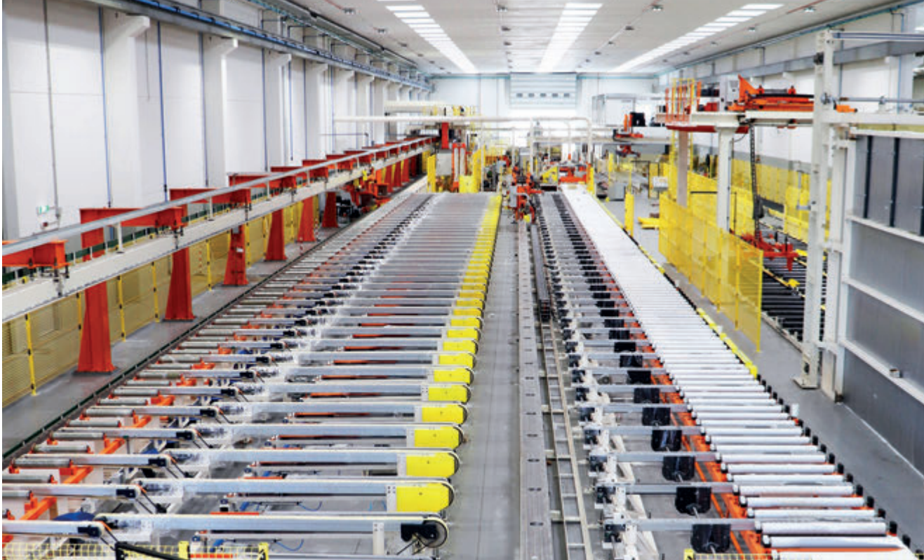
View of the extrusion bench of the new 2800-ton press
