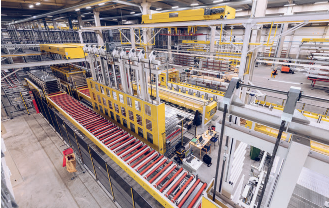
Automatic Profile Stacker with No Spacer Basket
