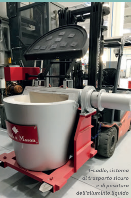
T-Ladle transport system with automatic T-Heater preheating device
