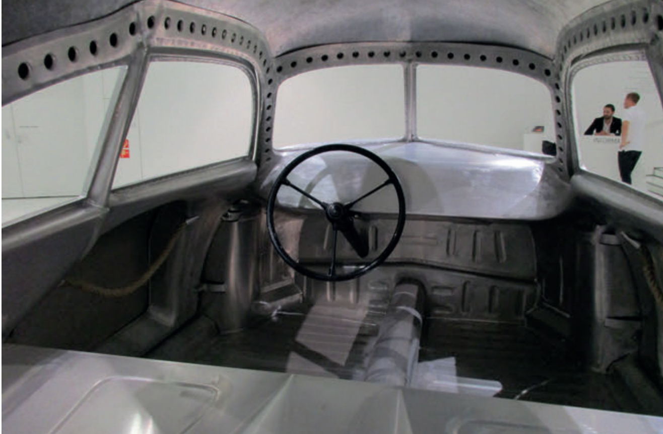
The inside of Typ 64's aluminium shell with clearly visible construction details (photo: ©Arnaud25/ Licence CC-BY-SA-3.0)
