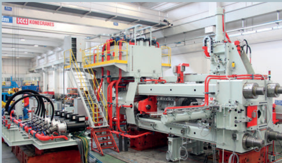
33 MN Front Loading Extrusion Press equipped with PE. Energy Saving System
