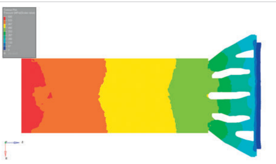
Figure 2: The press force required to extrude a defined billet length through the die is equal to the specific pressure at the dummy multiplied by the container cross section area. In this case study the value is equal to 61MN
