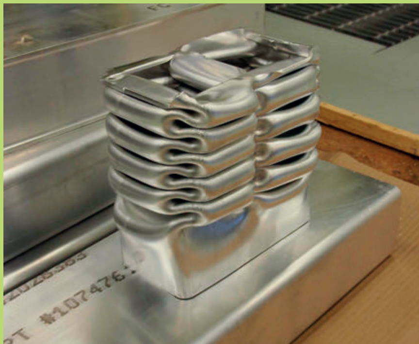
Structural aluminium extrusion after crash test
