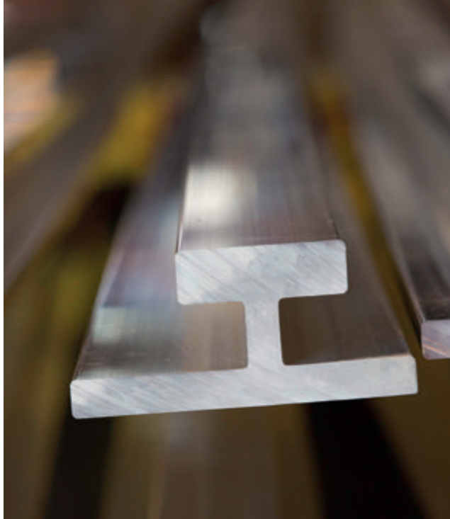
Figure 1: Section of an heavy extruded profile (courtesy of Constellium)
