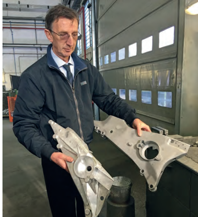
Enio Gritti with a traditional ribbed 3-mm gravity casting (left) and a new double-walled 2.6 mm casting
