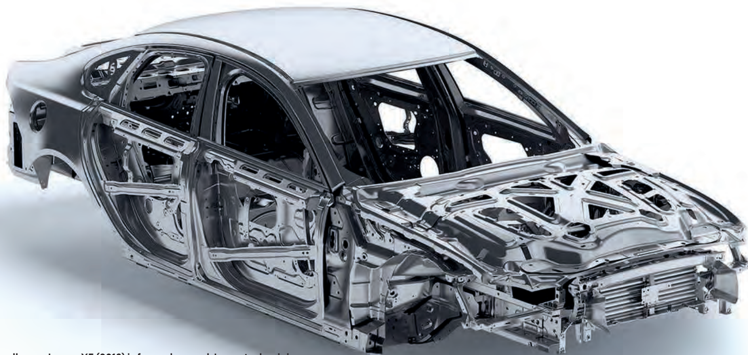
The all-new Jaguar XF (2016) is formed around Jaguar's aluminium-intensive architecture (Photo: www.netcarshow.com )
