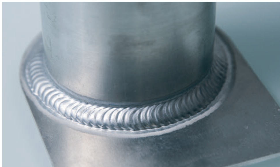
Aluminium component welded with the MIG "Active AL" process Componente in alluminio saldato con processo MIG "Active AL"
