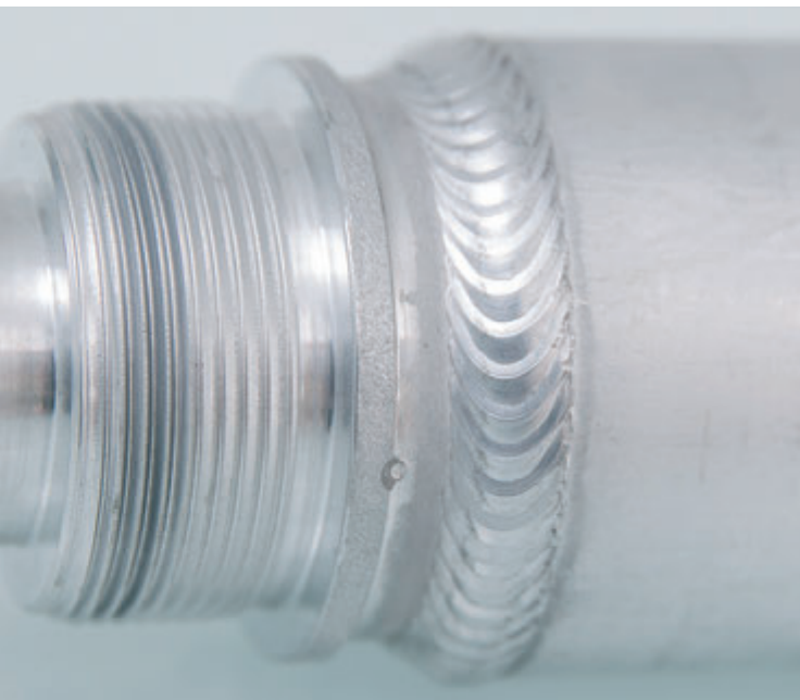
Aluminium component welded with the MIG "Active AL" process Componente in alluminio saldato con processo MIG "Active AL"
