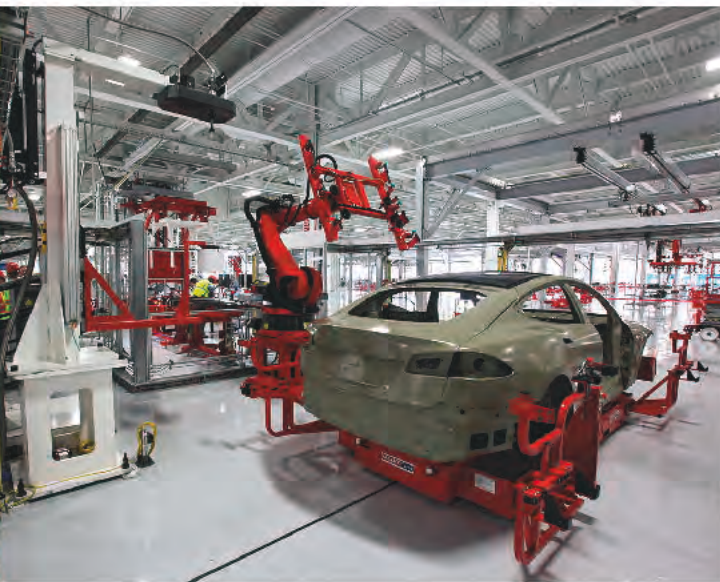
Figure 9: A Tesla Model S being manufactured at the Tesla Factory in Fremont, California; 98% of the Model S body is constructed from aluminium
